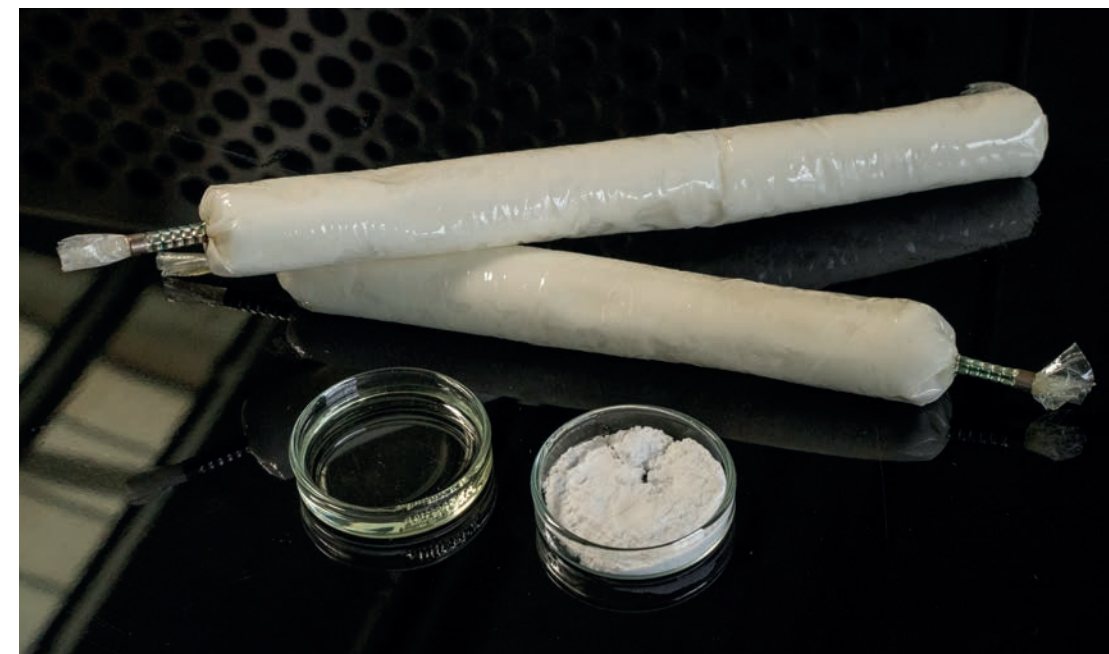
Suspensionsmolch aus Puderzucker und Rapsöl in möglicher Applikationsform. Suspension pig made of powdered sugar and rapeseed oil in possible application form.
