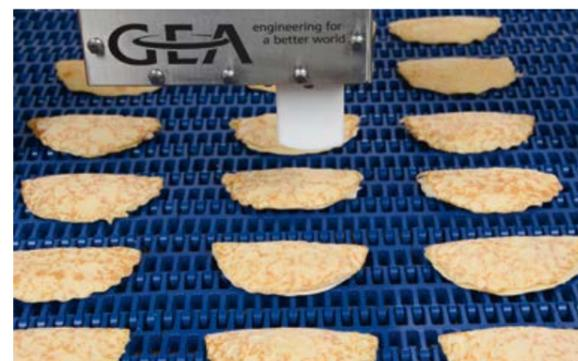
The new control system for spiral freezers is able to calibrate the freezer parameters through the continuous measurement of the level of frozenness of the product at the freezer exit. GEA has enhanced its control system to continuously monitor the level of crystallized water in the products and adjust the retention time, air temperature and fan speed to achieve the precise level of freezing required with the minimum of energy consumption.
